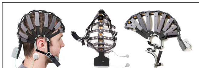
FIGURE 3 | Left: Subject wearing the headset. Reference electrodes are allocated on the side of the neck. Middle: View from the interior part of the headset with the structure that holds the electrodes. Right: Headset maintains its shape when not utilized. Picture, courtesy of Cognionics (Cognionics, Inc., San Diego, CA 92121).
