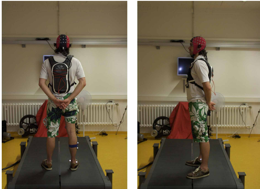
FIGURE 7 | ANT-Neuro eegosports™ wireless EEG system. Left: Posterior view: A study participant wearing the EEGOSPORTS WaveGuard EEG cap. The cap cable goes inside the backpack where it connects to the amplifier and Ultrabook. Right: Lateral view.
