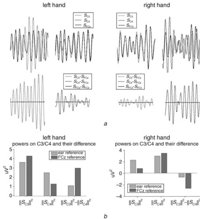
**Fig. 3** Examples of using FCz reference to enhance power difference between C3 and C4 during imagination of left and right hand movement
