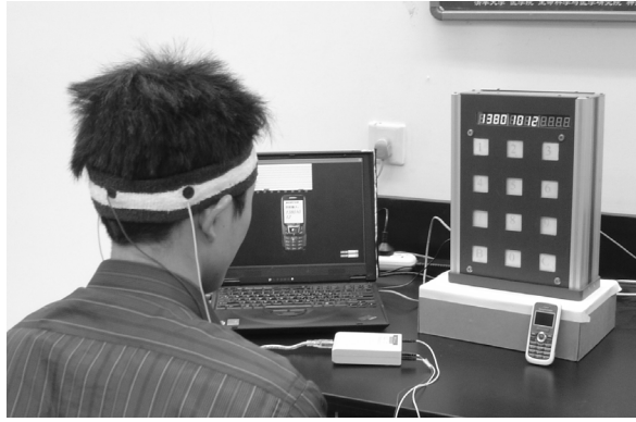
Fig.8. Application of the SSVEP-based BCI for making a phone call. The system consists of two-lead EEG recording hardware, an LED visual stimulator, and a laptop.
