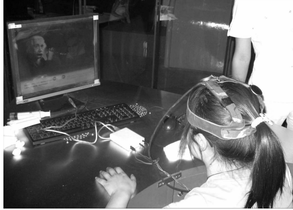
Fig.10. A player is playing a computer game controlled through a motor imagery based BCI. This system is available for visitors to the Zhengzhou Science and Technology Center in China.
