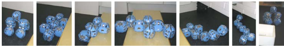
Fig. 23 Seven ATRON modules traversing an obstacle course, consisting of a step and a tunnel. When the car-like structure encounters the step, a cluster-walking behaviour is initiated. After the step, the cluster is transformed into a snake-like structure, to travel through the
