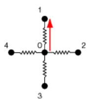
$\Delta V_1/R_1 + \Delta V_2/R_2 + \Delta V_3/R_3 + \Delta V_4/R_4 = 0 \implies (V_1 - V_0)/R_1 + (V_2 - V_0)/R_2 + (V_3 - V_0)/R_3 + (V_4 - V_0)/R_4 = 0$
