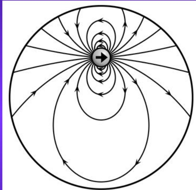
$$V = \frac{\vec{P} \cdot}{4\pi\sigma} \left\{ 2 \frac{\vec{R} - \vec{r}_0}{r_p^3} + \frac{1}{R^2 r_p} \left[ \vec{R} + \frac{\vec{R} r_0 \cos \varphi - R \vec{r}_0}{R + r_p - r_0 \cos \varphi} \right] \right\}$$
