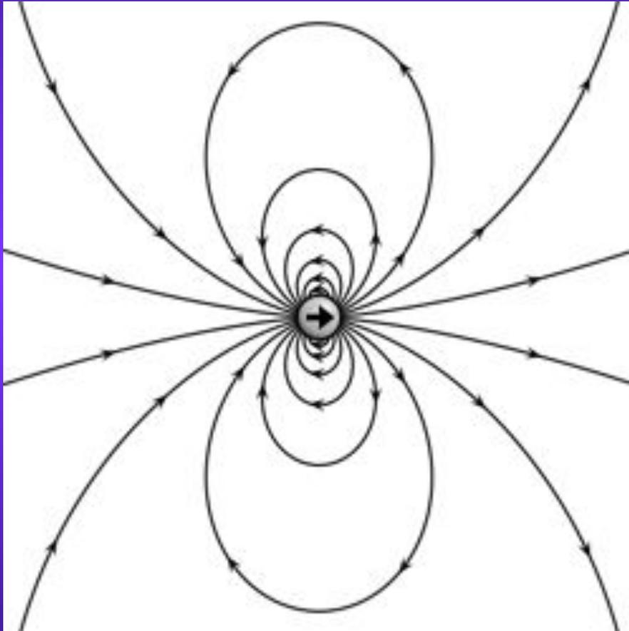
Field lines of a point dipole
